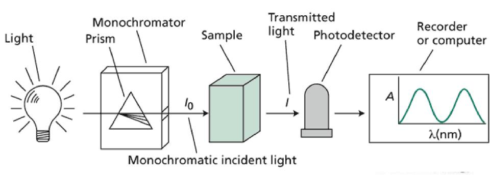
Optical Density Range (OD): As OD is a logarithmic scale, the accuracy of the reading is decreased if it is more than 0.9 and less than 0.1. Filter Choice: Commonly the most suitable colour of filter used to measure the concentration of a particular chromogen is complimentary to its colour as shown in table below:
